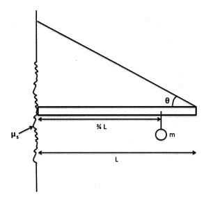
A log with mass 10 kg is held on a wall horizontally with the rope on a wall with finite static friction. L = 1m. Small mass m is hanging from the log at  $\frac{3}{4}$  L as drawin in the diagram. Hint: it is easier if you don't plug in the numbers until the end. I suggest keeping everything in T,  $\theta$ , g,  $\mu_s$ , M, and m, and then plug in the numbers.
