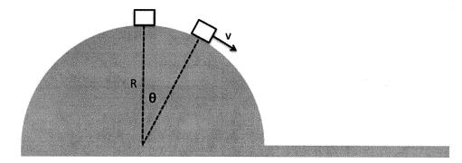
A mass with m=5 kg slides down a hemispherical shaped hill with a radius (R) of 1 m. There are no friction.
