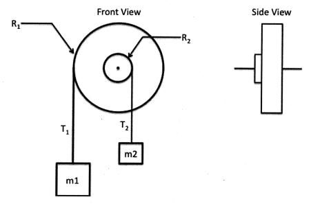
Two massive pulleys are glued together and set up with two masses.  $R_1=3m$ ,  $R_2=1m$ ,  $M_1=10$ kg, and  $M_2=5$ kg. Pulley's mass is 100 kg and its moment of inertia is given by  $\frac{1}{2}MR_1^2$  or  $\frac{1}{2}(100)\times 3^2=450$ kg  $\times$   $m^2$ .
