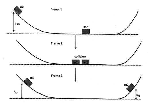
Three different frames above describe a sequence of events. In frame 1, objects start from rest. M1 accelerates down the slope and elastically collides with m2 in the frame 2. After the collision, both masses eventually each reach attain some maximum height. This question is about these sequences. m1 = 1 kg and m2 = 4 kg.
