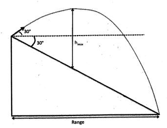
A projectile, with mass 10 kg, is launched with 30 degrees to horizontal on the slope, which is angled also at 30 degrees as depicted above. Initial speed of the projectile is 20 m/s. Gravity (9.8 m/s $^2$ ) points downwards on the figure as usual. Neglect consideration of air resistance.
